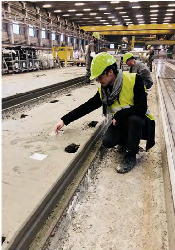
Install during fabrication RFID chips costs between 1-3 € per chip to install
